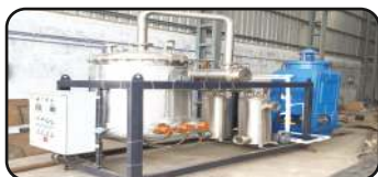
Electrical and Steam Jacketed Evaporator
